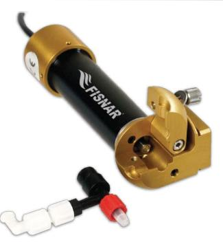
The RV5000DPM valve is designed for continuous operation where cleaning or refurbishment of a valve is not desirable. A disposable Delrin® auger screw is accessed through a hinged doorway and can be quickly replaced in seconds.
